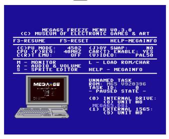
One feature to remember when playing games is the "(J)OY SWAP." This causes the two joystick ports to trade numbers. If you have a joystick in port 2 and you start a game that expects a joystick in port 1, instead of disconnecting and reconnecting the joystick, open the Freezer menu, press to swap the port numbers, then resume your game.
