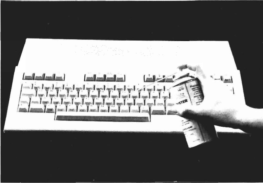
Fig. 1-9. Dusting the keyboard with compressed air.
