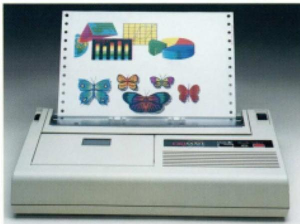
The Okimate 20 is sold with the Commodore Plug 'n Print Kit. This revolutionary ribbon transfer color printer has a 24-element thermal printhead that can print beautiful copies of Commodore 64/128 screens. It prints text at 80 characters per second in standard mode, 40 cps in near-letter-quality mode. Page widths are 80 columns in standard mode or 132 columns in condensed mode. Other print features include expanded, italics, fine print, underlining, superscripts, and subscripts.
