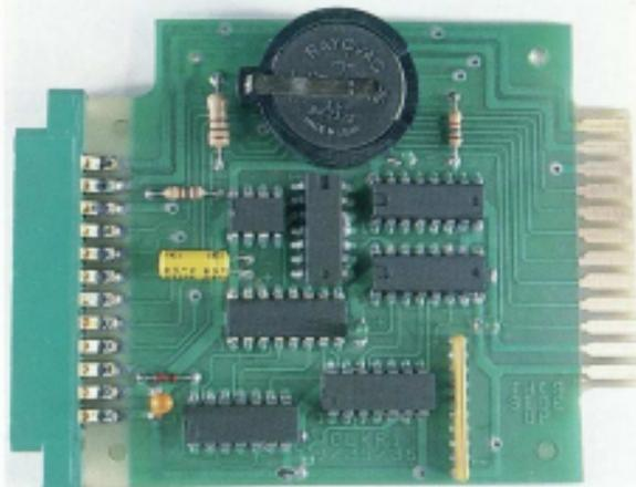
"THE RIGHT TIME" is a battery backed real time clock-calendar for your C-64 or C-128 (all modes) that keeps the correct time and date even when the computer is turned off! The clock is plugged into the user port, but still allows full use of the port by any other peripheral. Software for reading and setting of the real time clock is included. Connectors are gold plated for dependability. "THE RIGHT TIME" is available at dealers nationwide.
