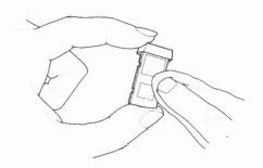
10. When cleaning, place the printhead on a flat surface with the protective cap off the edge of the flat surface. Do not exert too much downward pressure near the center of the assembly.
