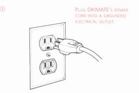
Do NOT use an adapter which ignores the ground, or your printer could be damaged.
