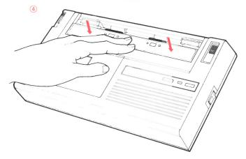
Make sure the top of the sheet is even with the paper window. Printing will start 1/2 inch below this point.
