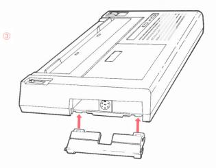
Engage its slots with the module's metal tabs.
