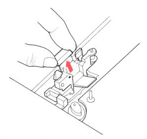
**NOTE:** Always handle the printhead by the protective plastic cap or along its sides. Do not touch the thermal surface.
