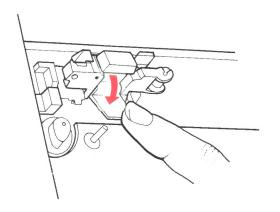
7. Grasp the blue cap attached to the printhead, then lift the printhead out of its assembly.
