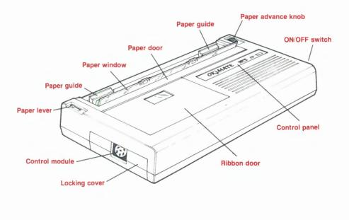
The CONTROL PANEL buttons let you activate the printer and control print darkness. The READY light tells you the printer is ready to print, and signals you if there's a printing problem, such as running out of ribbon or paper.
