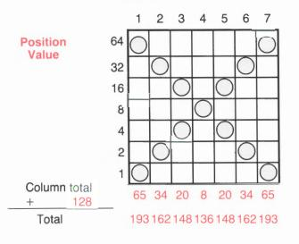
**NOTE:** To be compatible with Commodore graphics, the graphic data must be sent in 8-bit form. Therefore, the 8th bit, 128, must be added to the total for each column. This 8th bit will not be printed.
