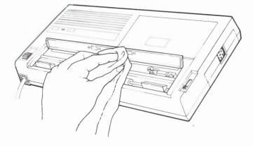
Clean the OKIMATE printhead when you change the ribbon, or whenever you notice the print fading or missing print dots.
