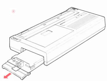
While holding the cover at its edges, gently pull out the module.
