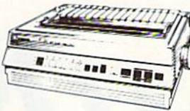
The 1180 by Panasonic offers you more than what you might expect in a low cost printer. With multiple paper paths, versatile paper handling, and front panel programmability through the EZ Set Operator panel. The 1180 also features Near Letter Quality (38 cps) and Draft (192 cps) plus crisp, clear graphics.
