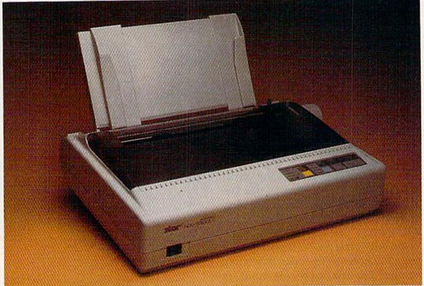
The Star Micronics NX-1000C Multi Font includes four onboard fonts that are selected from the front control panel.
