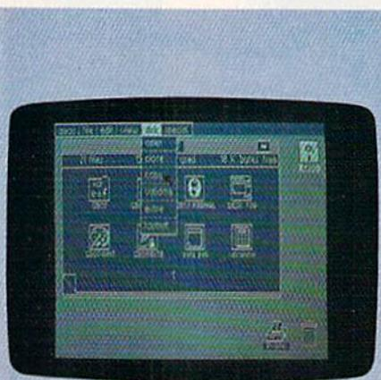
The copy feature has been selected by pulling the disk options menu down from the Command Bar.
