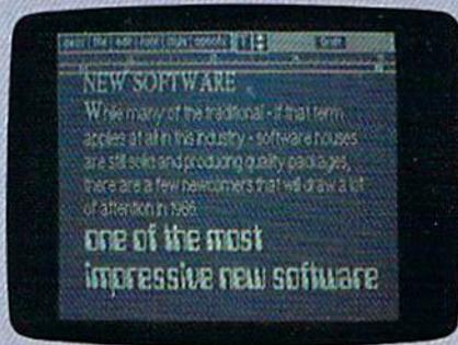
*geoWrite* offers a wide choice of different sizes and styles of text. Note the margins and tab set on the ruler at the top of the screen. This is half-width mode.
