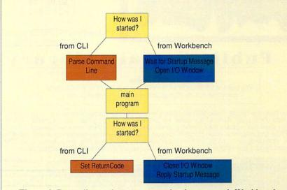
Figure 1. Depending on how a program has been started -Workbench or CLI- a program needs to do certain things, both as it starts and as it terminates.
