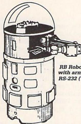
**RB Robot with arm and RS-232 (TINY BASIC)**
