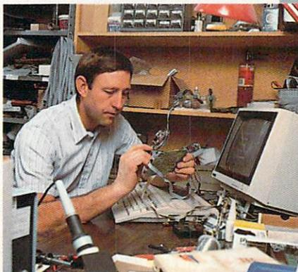
Final test and inspection of B100 interface using another B100.
