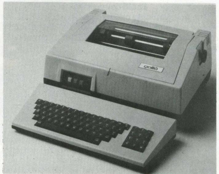
*The Gallid Superwriter II 80/132 column dot matrix printer, suitable for most computer installations*
