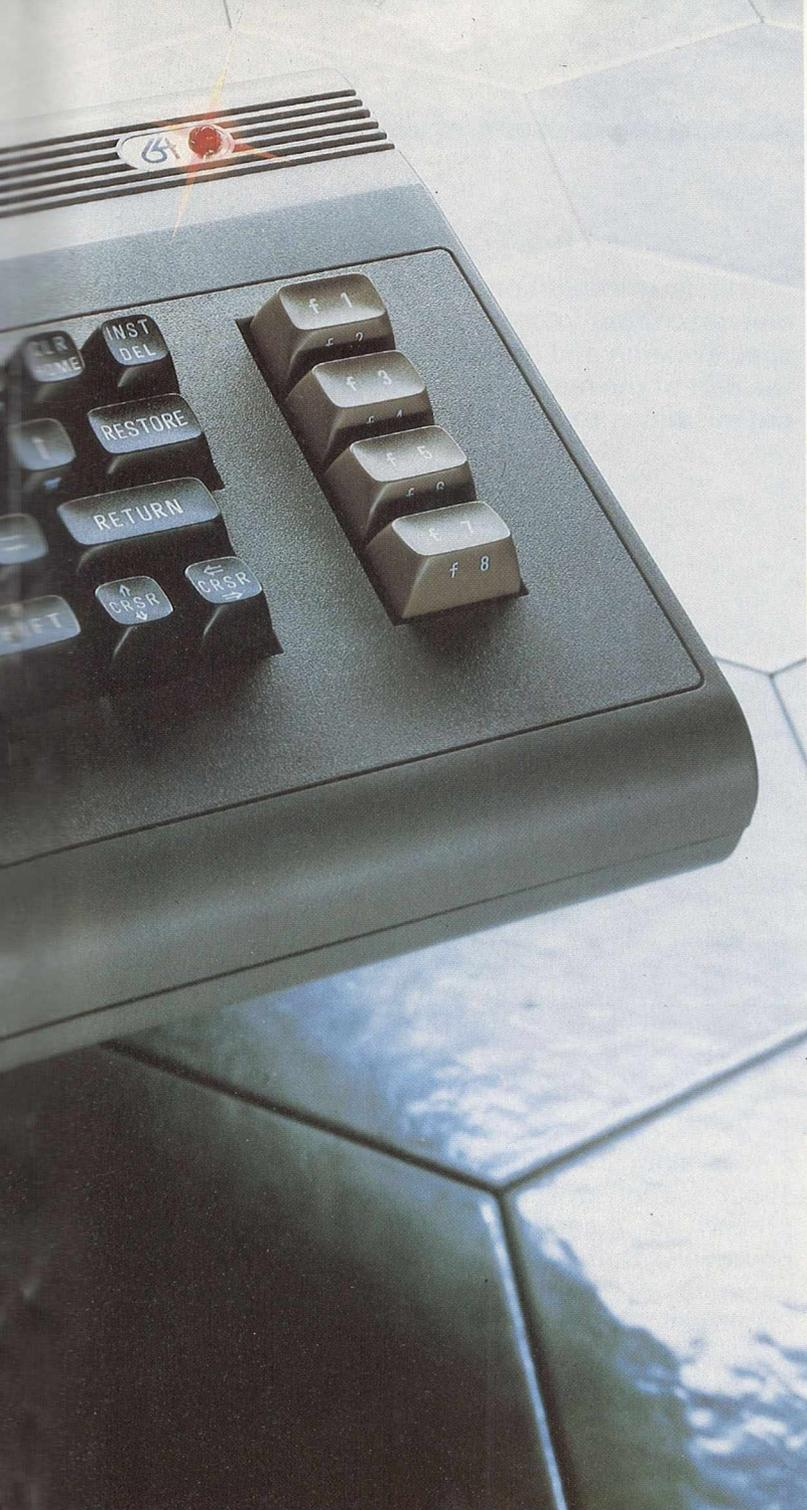
full alpha numerics with upper and lower case letters, all available directly from the keyboard and displayable in normal or reverse video in any of 16 colours.
