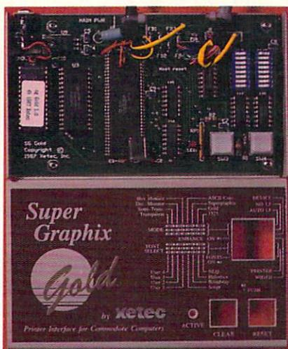
*Inside Super Graphix Gold lurks (left to right) 32K of ROM, 32K of RAM, and an 8 bit 6303 microprocessor. The 5V regulator is at upper left. Switch settings are clearly labeled on the cover.*
