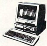
512K RAM Computer Keyboard 360K Floppy Drive 4.7-7.16 MHz. 12" Monitor 8088-2 Processor
