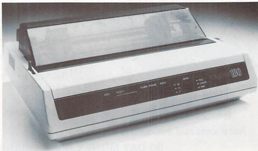
*The Okidata 180 offers pushbutton control of line/form feeds, print mode and pitch selection, etc. on its front panel. READER SERVICE NO. 217*
