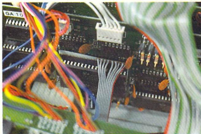
*Installation of 21 Second Backup in an SX-64. Access to the VIA chip is more difficult than on the 1541 (below).
