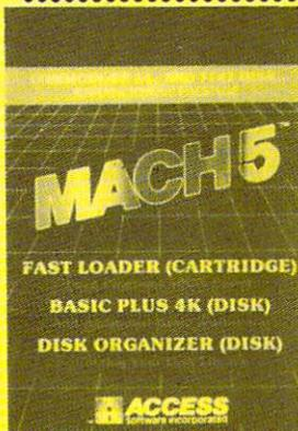
**Mach 5** — Plug Mach 5 into the cartridge port and turn on the computer, the cartridge works automatically to load programs up to 5 times faster than normal. Loads 99% of all software, even copy protected games. Works with all popular printers. Will list directories without disturbing programs in memory. Commands such as LOAD, SAVE, OPEN etc. are executed with one keystroke. More features than most other "fast loaders". Does not disturb RAM. (Cart.) List \$34.95. **Sale \$19.95.**
