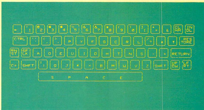
mode on the 128 and wish to return to QWERTY mode, just hold down the RUN STOP key and hit the side reset button. When you are dumped into the monitor, hit 'X' and RETURN. If you do accidentally hit RUN STOP/RESTORE on the 64 and want to return to Dvorak mode without rerunning the program, you can simply type POKE1,53 and press <RETURN>.
