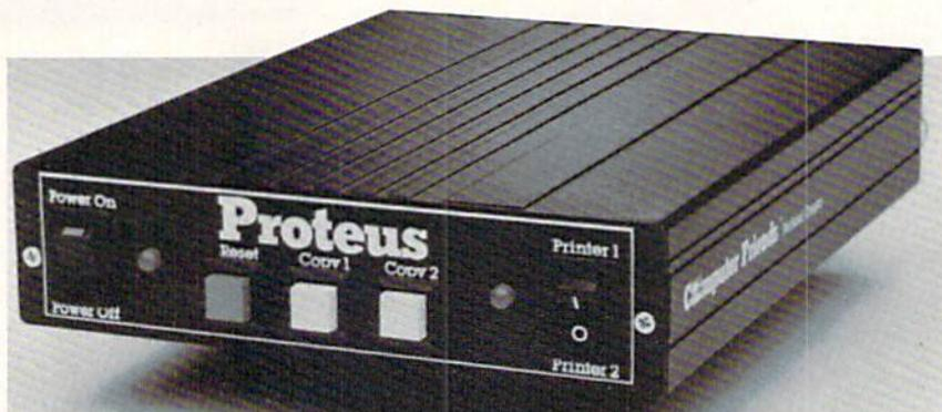
**Proteus buffer/data switch: connect two peripherals to any computer.**
