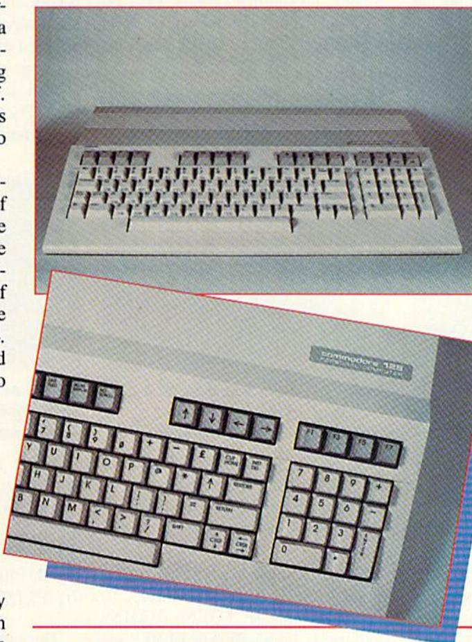
*Top: all 92 keys of the C-128. Main section nearly duplicates the C-64. Bottom: closeup showing numeric keypad.*
