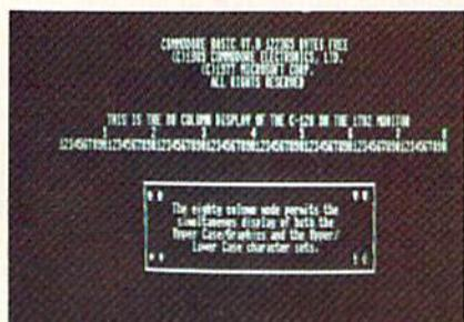
An 80-column display using the 1702 color monitor (see sidebar, p. 32).
