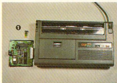
The Okimate 10 Color Printer, side by side with its attendant ① user-replaceable thermal print head and ② Plug 'n Print module.
