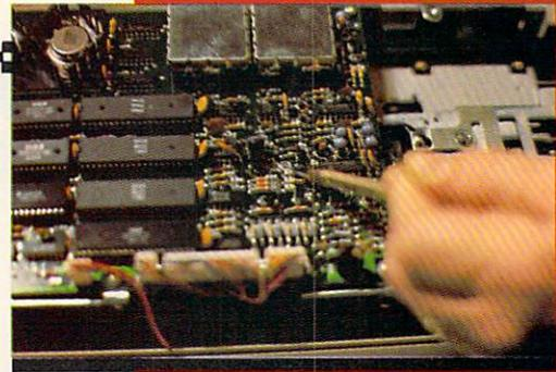
**FIG. 5** *Location of device # jumper on current models of the 1541.*
