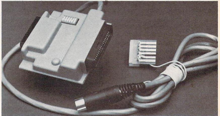
Card/?PS universal parallel/serial interface uses Commodore print format. **READER SERVICE NO. 80**
