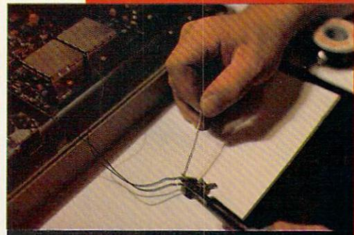
**FIG. 7** *Soldering ends of hookup wire onto two switch terminals.*
