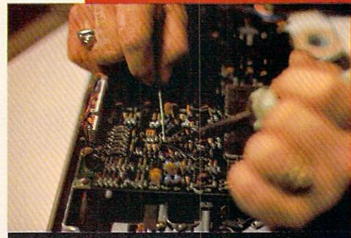
**FIG. 6** *Soldering wires to device # jumper. Work carefully here!*
