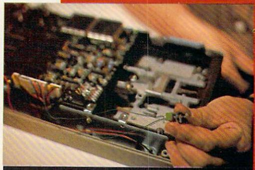
**FIG. 8** *The completed solder connections to jumper and switch.*
