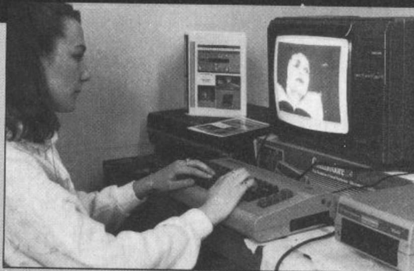
CRL, A FIRM ALREADY WELL KNOWN for its software, has now moved into the peripherals market with the launch of the Video Digitiser Module for the C64.
