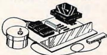
STEPPING MOTORS are extremely precise specialized motors. With the aid of the computer, the shaft can be rotated any number of revolutions to the exact position you want. Very simple poke commands pulse this geared down, high torque motor 1.8° for 200 steps per revolution.
