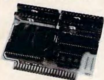
16-channel A/D converter & 1-channel D/A output; 16 high-current discrete outputs.
