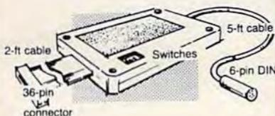
Works with all centronics type parallel matrix & letter printers and plotters—Epson, C.Itoh, Okidata, Nec, Gemini 10, TP-1 Smith Corona, and most others. Hardware driven; works off the serial port. Quality construction: Steel DIN connectors & shielded cables. Has these switch selectable options: Device 4, 5, 6 or 7; ASCII or PET ASCII; 7-bit or 8-bit output; upper & lower case or upper only. Recommended by PROFESSIONAL SOFTWARE for WordPro 3 Plus for the 64, and by City Software for PaperClip.
