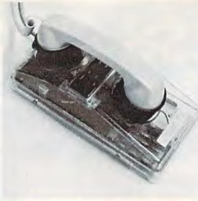
*An example of an acoustic modem, with its rubber cups fitting tightly on the telephone handset.*
