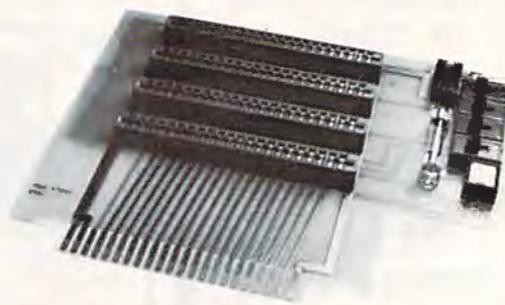
The CP VIC-20 Expander is the one you have been waiting for. It incorporates all the features you've ever asked for. For only \$64.95, the CP VIC-20 Expander gives you: Four high quality connector slots with keys; Gold plated contact fingers for positive and long-lasting connection; On board master reset button; Four convenient ON-OFF individual slot control switches; External power supply hook-up provision with two-way power switch and overload fuse block.
