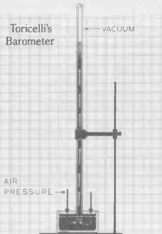
causing the mercury in the glass tube to rise. When the pressure was low, the mercury in the glass tube fell.
