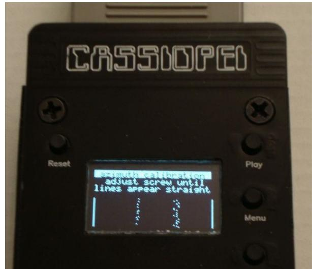
Switch off your CBM computer, connect the datasette to your Cassiopei, press the play, wind or rewind button and switch on the CBM computer. The Cassiopei will detect the datasette (because the sense line is active caused by the pressed play, wind or rewind button) and will show a different screen. This is the .TAP creator mode (a.k.a. the backup/restore mode).
