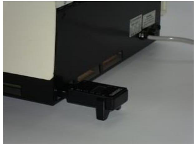
As the image above demonstrates, the PET/CBM 2000 and 3000 series require the use of an additional stand. You can attach this by removing the back cover of the Cassiopei and then slide the stand gently over the cassetteport connector, then replace the back cover.
