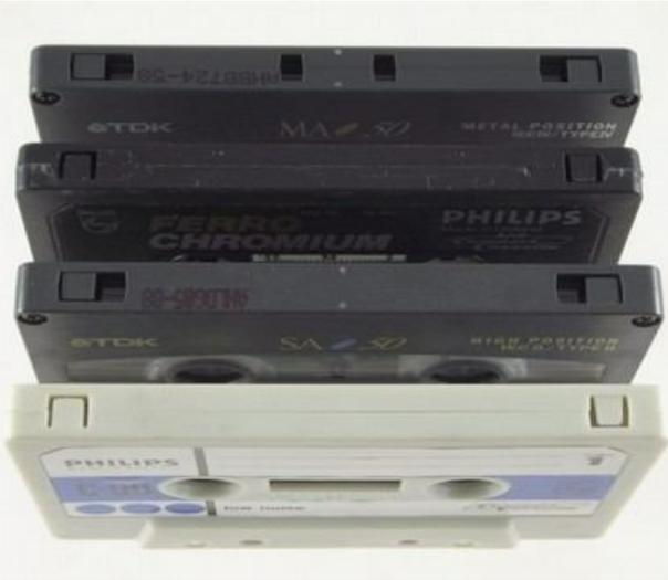
**Type IV:** tapes referred to as “metal”, it can be identified by the wider write protect tab hole and extra holes in the center of the tape.
