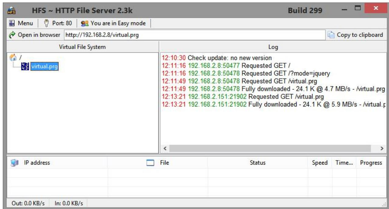
Above you see that the file “`virtual.prg`” has been added to the “root”, it was done using the menu→`Add_files...` function. The port value is shown on the top of the screen and is default set to 80, a value which I prefer because this way I can quickly test the connection using my webbrowser without having to enter (and remember) the port address.
