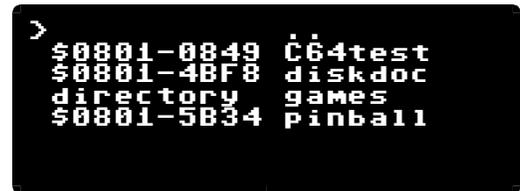
The only way to exit this menu is by selecting a file, if for some reason there are no files stored onto your SD-card then the only way to exit is by pressing the “Reset”-button on the Cassiopei.
