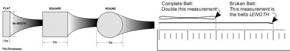
When I (the writer of this manual) replaced the belt in my 1530 dataset, I measured that the thickness of the new belt was 1mm x 1mm (in other words, a 1mm square belt).
