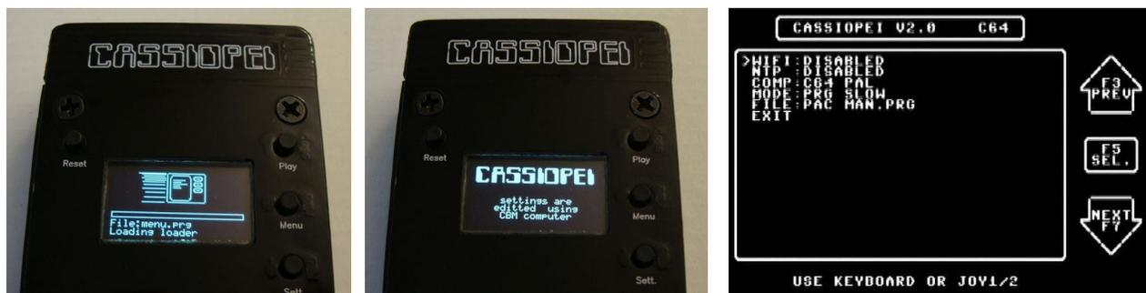
Use the keys as indicated in the screen to browse through the menu. When exit is selected (in combination with exit & save settings) the current selection is saved to the settings file and executed, which saves the user the trouble of typing LOAD again.
