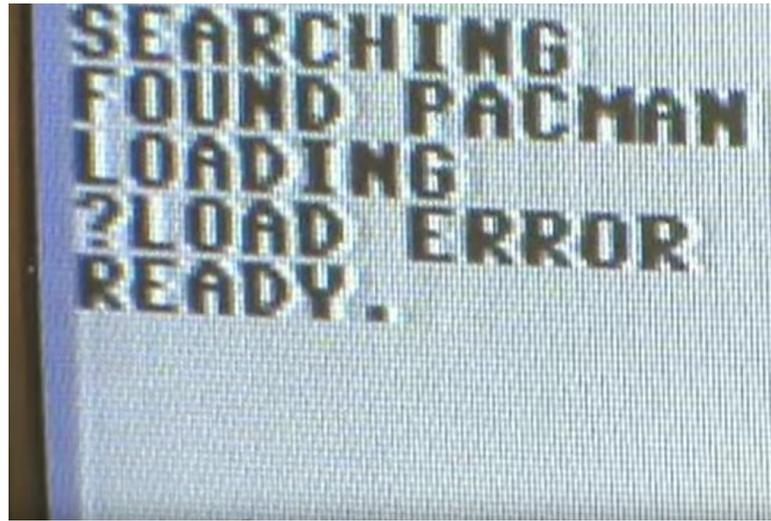
datasette (and any other kind of tape drive used for home computing in the 80's) is tapehead alignment, also referred to as azimuth. Make sure that your tapeheads are aligned properly.
