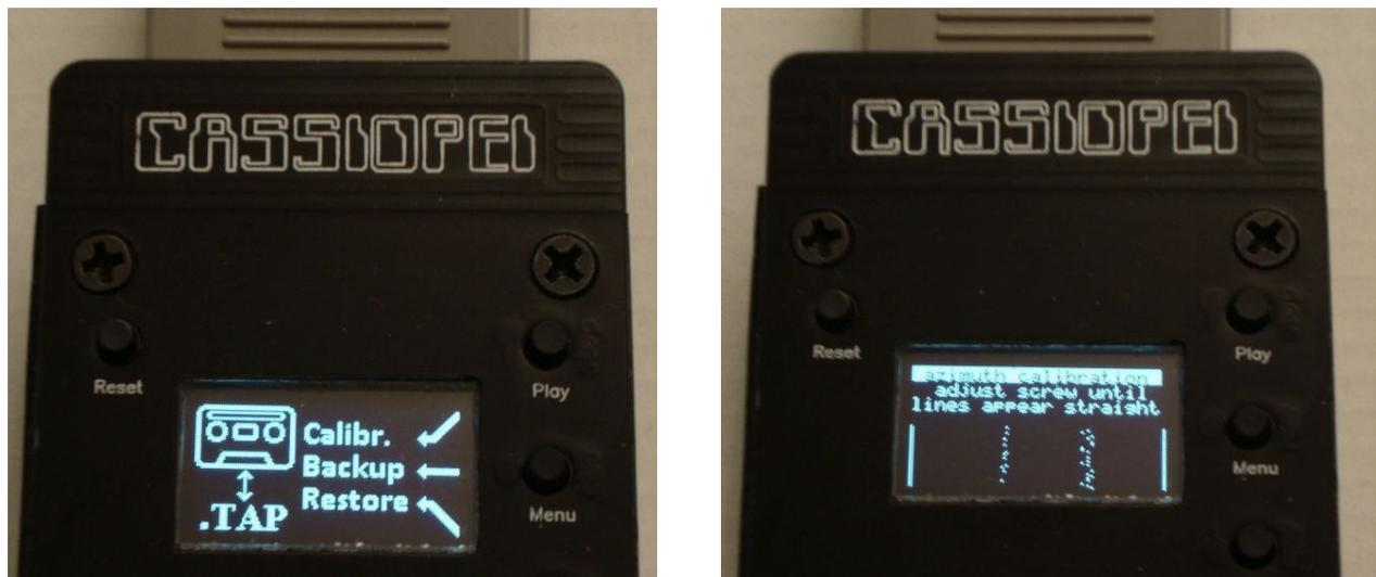
Switch off your CBM computer, connect the datasette to your Cassiopei, press the play, wind or rewind button and switch on the CBM computer. The Cassiopei will detect the datasette (because the sense line is active caused by the pressed play, wind or rewind button) and will show a different screen. This is the .TAP creator mode (a.k.a. the backup/restore mode).
