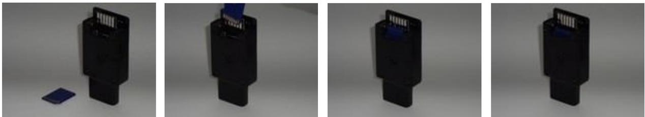
This SD-card has to be properly configured, with the right folders and the right files. The Cassiopei uses an SD-card that must be formatted according to the FAT-16 (which is called FAT in MS Windows) or the FAT-32 format. If an SD-card is not supplied with the Cassiopei or if you want to alter the contents of the card, please consider the requirements as described below.
