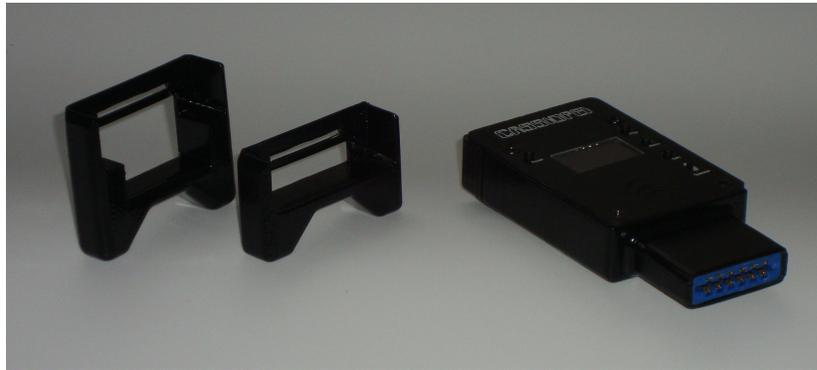
In order to attach a stand to the Cassiopei, remove the back cover and slide the stand with the smallest slot gently over the cassetteport connector.
