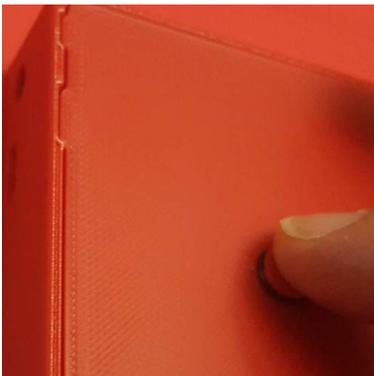
7. Press the peg into the cartridge very gently, which will allow the O-ring to settle. The peg should be flush. (If it is not, try tightening the screw.)
