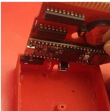
3. Insert board as shown (just deep enough so that the jack fits into the groove). Be careful with the LED, as it can easily get bent.
