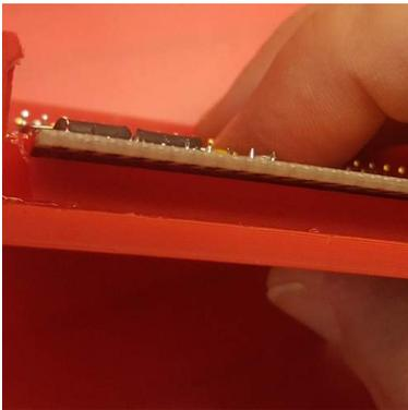
5. The board should fit snugly against the edge of the case and lay completely flat.
