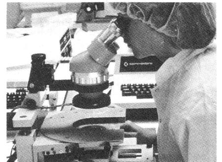
New RAM and ROM memory circuits are checked for technical accuracy.
