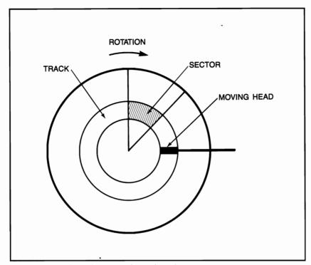
Figure 1.6: Tracks and Sectors of a Disk Surface
