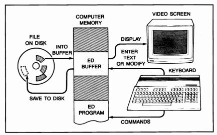
Figure 5.1: The Edit Buffer in Relation to the Disks, Keyboard, and Video Screen
