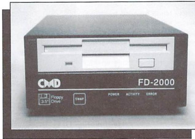
drive mechanism, and is the traditional IBM clone beige color. The front panel contains 1 switch and 3 LEDs in addition to the customary manufacturer logo and drive model number. The LEDs are labeled "Power", "Activity", and "Error". Turning the unit around, we see the back of the unit is pretty simplistic as well. Two serial bus connectors are provided, as is a connector for the power supply and a power switch.
