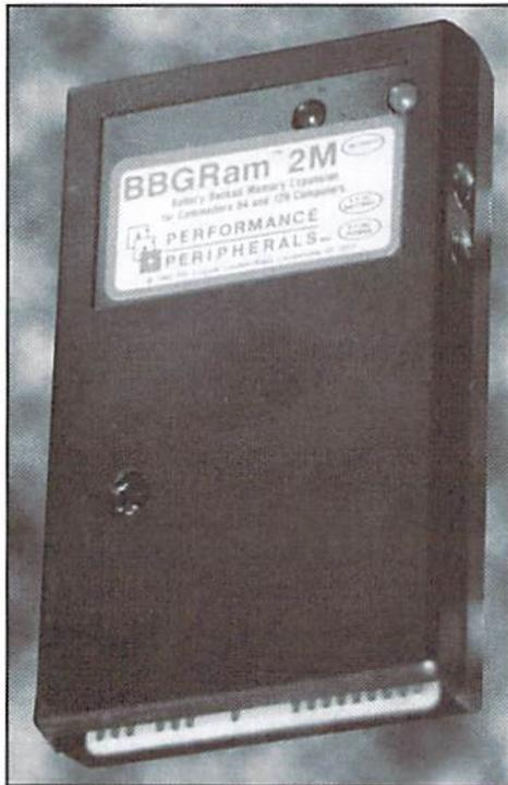
computer is shut down via the power supply and battery backup. The unit is shipped with a utility disk which includes a BBGRAM tester, a few diagnostic programs, and a number of GEOS support utilities.
