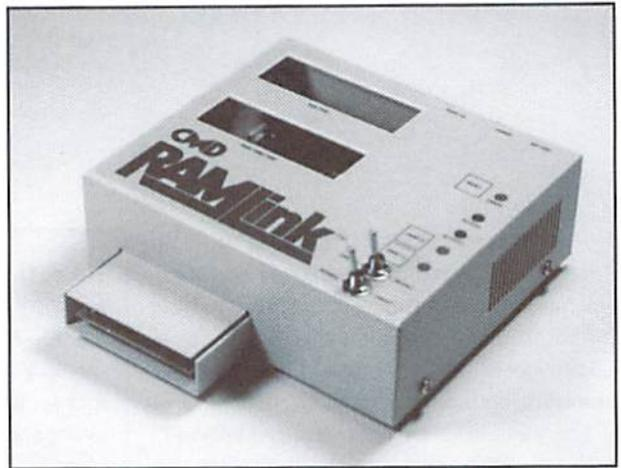
RAMLink disable switch. In the back of the RAMLink unit rests a parallel port, offering CMD HD Series hard drive owners faster access. The RAMLink comes standard with a small power supply and has a battery backup option. Both of these plug nicely into the back of the cartridge. And finally, the RAMLink features a number of LED's to reflect its current state.
