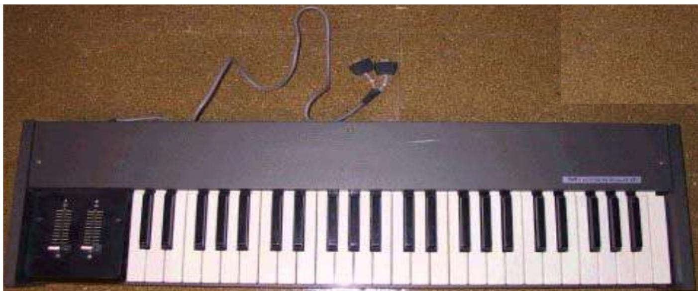
The keyboard also has two analogue sliders that are assignable (more on this later).
