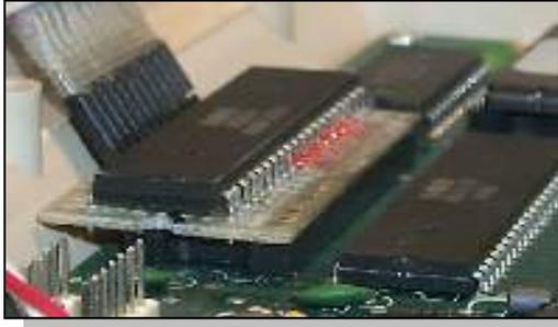
[1571 low profile parallel cable adaptor, top view,
