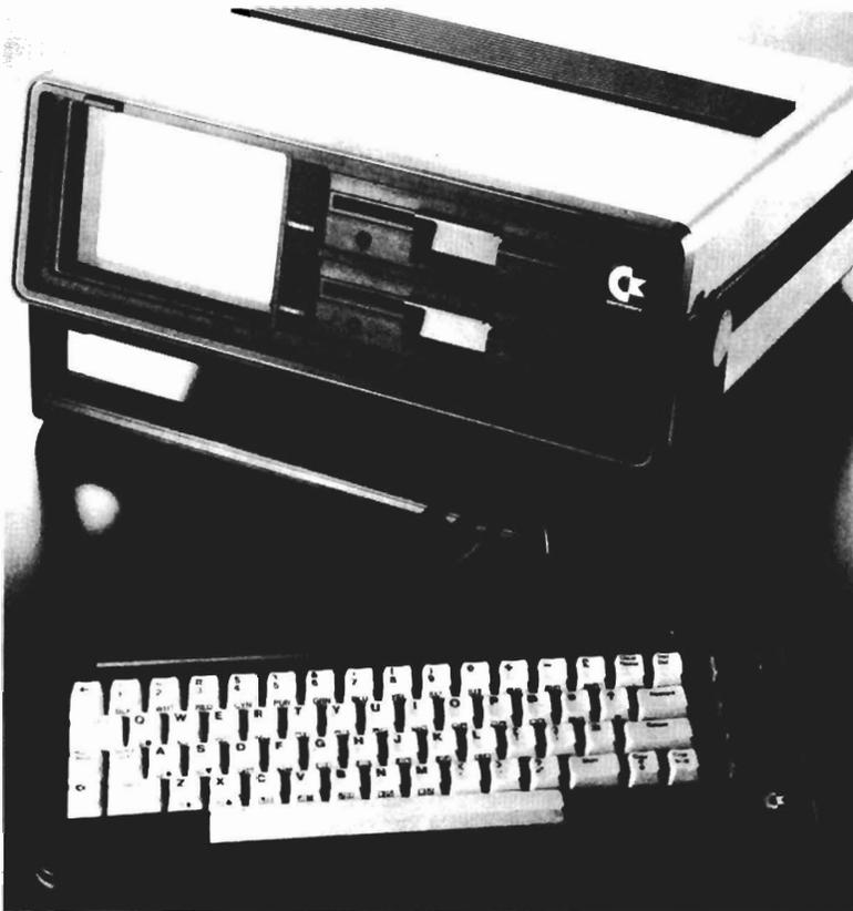
To the left: The Commodore portable Executive 64, weighing 27.6 pounds, travels easily. It has 64K RAM, a built-in, five-inch monitor, and floppy disk drives with 170K capacity.
