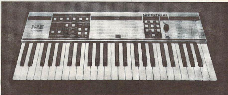
The MAX keyboard from Sequential Circuits is a MIDI-keyboard especially designed to operate with computer equipment.
