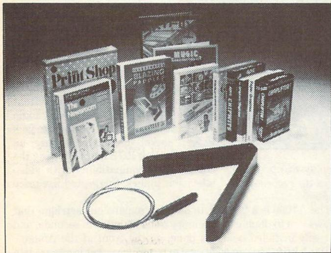
The 'Space Pen', from Soniture Inc., is a two-dimensional or three-dimensional input device for the Commodore 64 and other computers. In its 2-D mode, it is compatible with existing joystick and touch tablet software.
