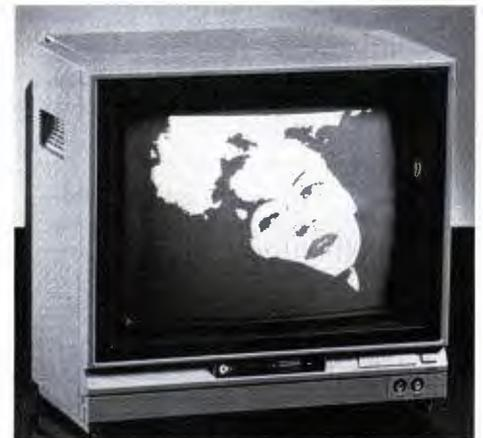
The new 13 inch monitor—designated the CBM 1701—will retail for \$299.95 and was especially designed for use with the COMMODORE 64 and VIC 20 computers. The monitor accepts a standard 75 ohm composite video signal or a "Commodore" video signal with separate provisions for luminance and chrominance signal input as well as audio input.
