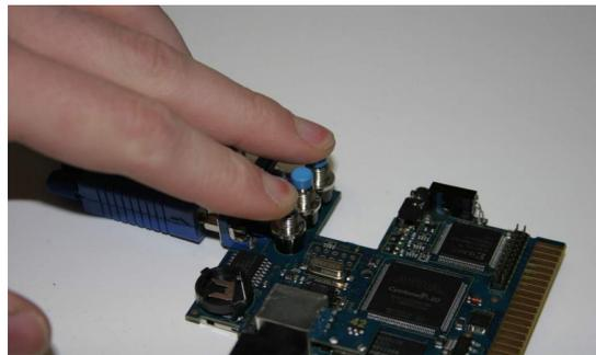
Then release the right (reset) button, but keep on holding the left button. As the last step, release the left button:
