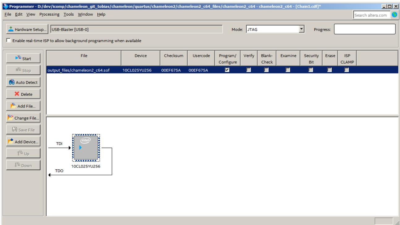
Finally, click Start, and the project should be uploaded to the FPGA.
