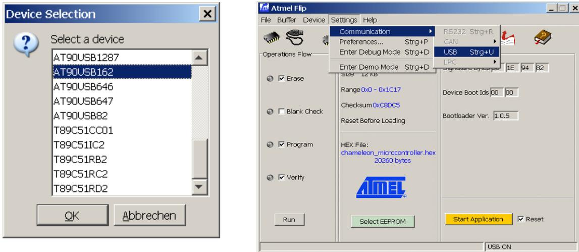
Now load the micro-controller hex file by clicking on file->Load hex file. The final step is to click on the “Run” button within FLIP (at the bottom left of the window) and watch the program do its magic. After programming the micro controller, FLIP will indicate the successful steps with a green light next to the action tags:
