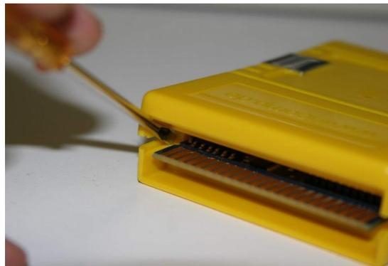
With the opening in the Chameleon case for the mini-DIN connector, the left half of the case top is fairly weak. We therefore recommend to open the right side of the case first:
