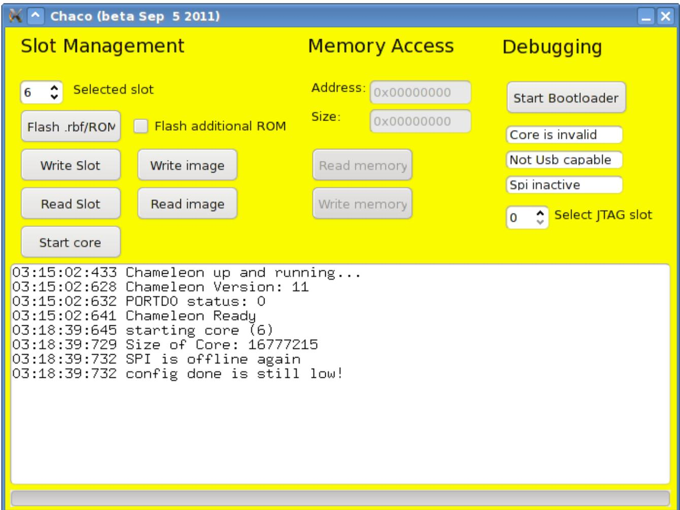
The error message in the window reflects what you should see on Chameleon: The red LED should blink seven times, then pause, then start over with blinking.
