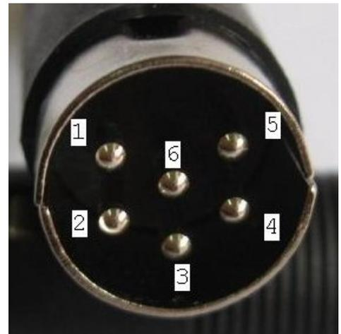
Connection CN1 to CN2 is a 5-core shielded AWG26 cable:
