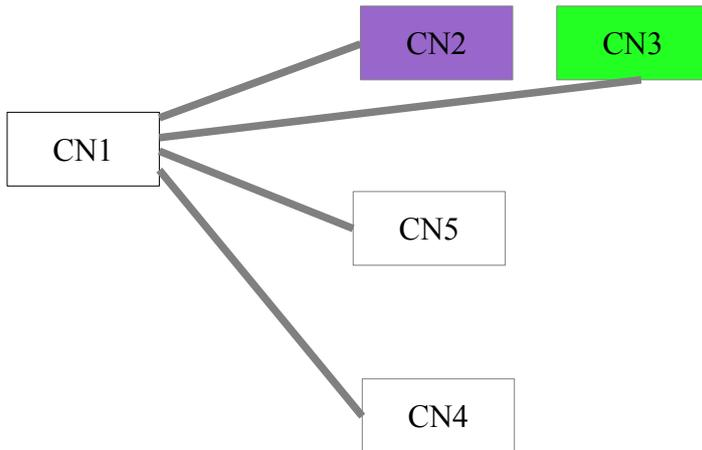
Connection CN1 to CN2 is a 4-core shielded AWG26 cable, length 200mm:
