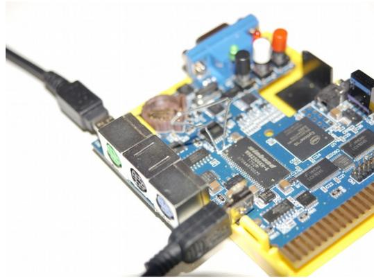
Now make two USB connections to your PC and switch on the PC. Then place the micro-controller into de-brick mode with the following combination of button presses. Press and hold the left button, then press the right (reset) button:
