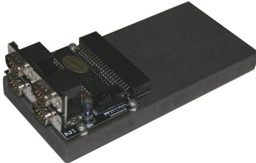
Both keyboard connectors are keyed, which means that they have a missing pin in order to help you finding the correct orientation of the connector. However, the A500 keyboard connector is not always keyed, so you have to take a close look at the colours. The black wire of the A500 keyboard is marked next to the connector. Wrong connection may destroy both, the docking station and the keyboard! Better double-check before you apply power to the unit.
