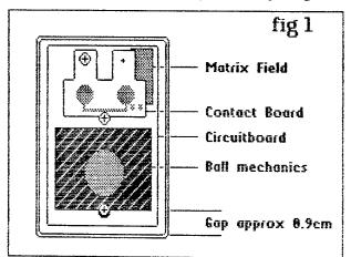
The upper casing should now be placed in a safe place. We are now looking at fig 1
