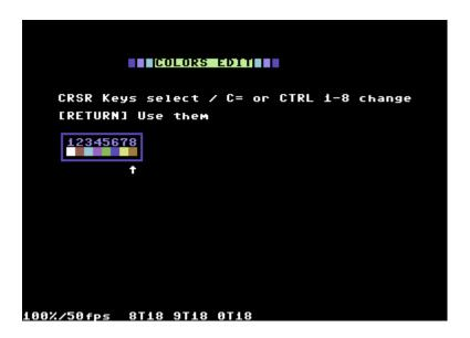
To change the eight colors use Cursor Keys to move the selection Pointer and enter your colors by pressing <CONTROL> + <2> till <8> or <CBM> + <1> till <8> for the built in colors. Press <RETURN> to quit editing and save the file to disk afterwards. Keep in mind the Background Color is always set to Black. To avoid Textlines that the User can't see in his Terminal Program, the use of CTRL+1 (black) is denied in this Editor.
