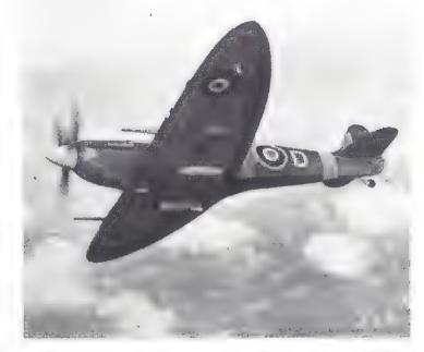
when the G-forces caused fuel to flood the carburetor. To prevent Bf 109 pilots from taking advantage of this, British pilots would execute a half roll and dive, which kept the Spitfire's engine running. The carburetion flaw was later corrected, and the Spitfire would go down in history as perhaps the best defensive weapon of the war.
