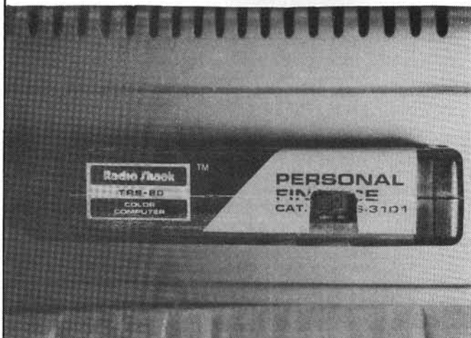
Photo 4: Program Pack installed; note case cutout and protruding defeat switch handle.
