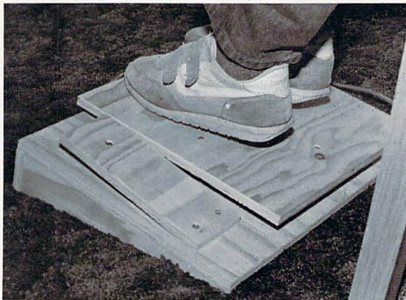
Figure 5 Foot joystick in action
