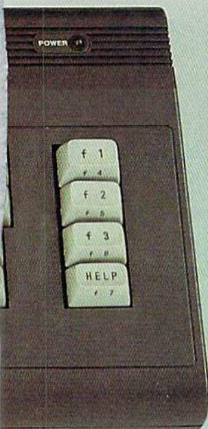
The Commodore 16 is a 16K computer (12277 bytes free) with BASIC 3.5 and a built-in monitor (TEDMON). BASIC 3.5 contains over 110 commands, statements and functions and TEDMON contains an additional 16 commands. Although this is a new line of computers, Commodore has kept it compatible with all of the major Commodore 64 peripherals (monitors, disk drives and printers).
