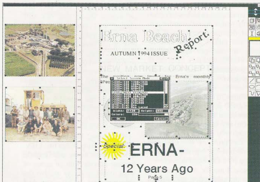
Professional Page now runs in 256 colours on a graphics card screen, but this gain comes at the expense of 16 colour operation, leaving only black and white for unexpanded Amigas.
