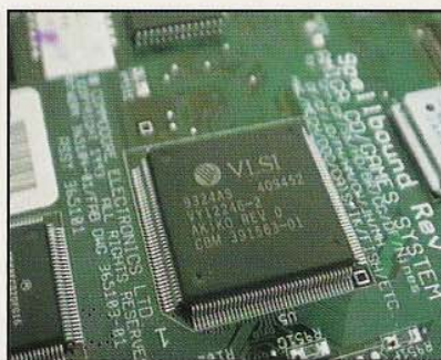
New VLSI chip handles I/O plus conversion from PC to Amiga graphics
