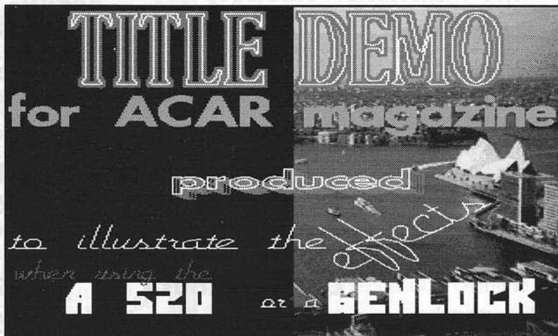
Picture 2: In contrast to the A 520, a genlock allows replacing the background (colour 0) with live video. Titles with different fonts and effects can be created even by cheap or completely free non-commercial software, as in this example
