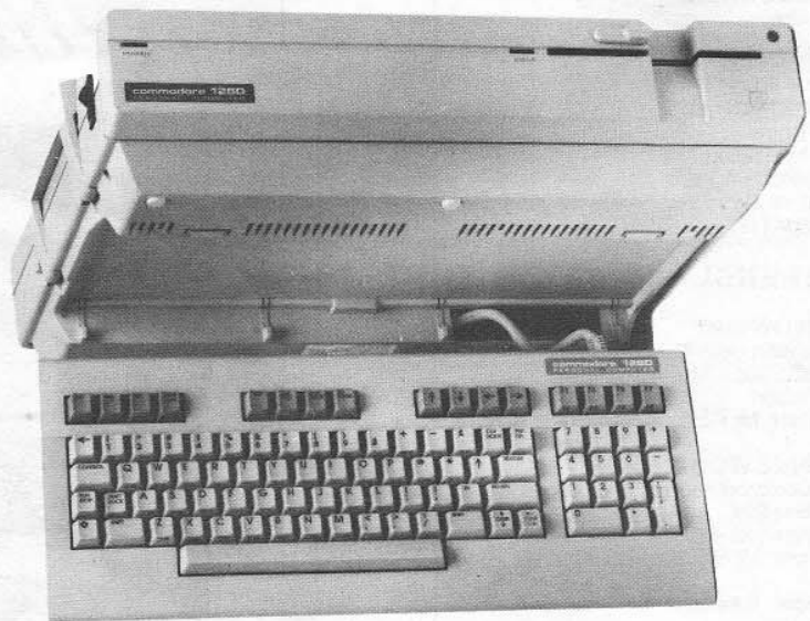
The Commodore 128D has a slimline keyboard which clips into the back
