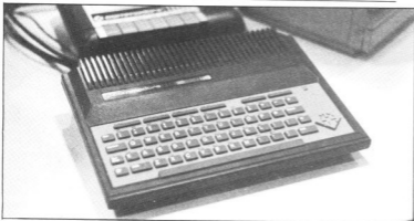
This is a little beastie you definitely won't see in any British shops. Called the Commodore 116, it's really a Commodore 16 with a small Plus/4-style case and 'chiclet' keys rather like the old Spectrum. Apparently the machine was to be marketed only in Germany where it hasn't gone down very well. Yet another black mark for Commodore's marketing strategy.
