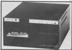
In the picture is a new mini-Winchester disk (uses a 5 1/4-in non-removable hard disk) for the CBM 600X. It stores 18 or 36 megabytes, has an integral tape streamer for backup, and includes enough intelligence to provide for multi-user operation — up to 18 users can attach to it, up to 40 relative files can be opened at the same time, and file access protection is built in via disk status procedures. It hauls from DMI Computing — details from 021-396 4648.
