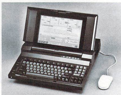
The Yamaha C1 Music Computer orchestrates 11 MIDI ports and a megabyte of memory.
